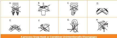
Rollout: A process by which a snap hook or carabiner unintentionally disengages from another connector or object to which it is coupled. (ANSI Z359.12-2019)
